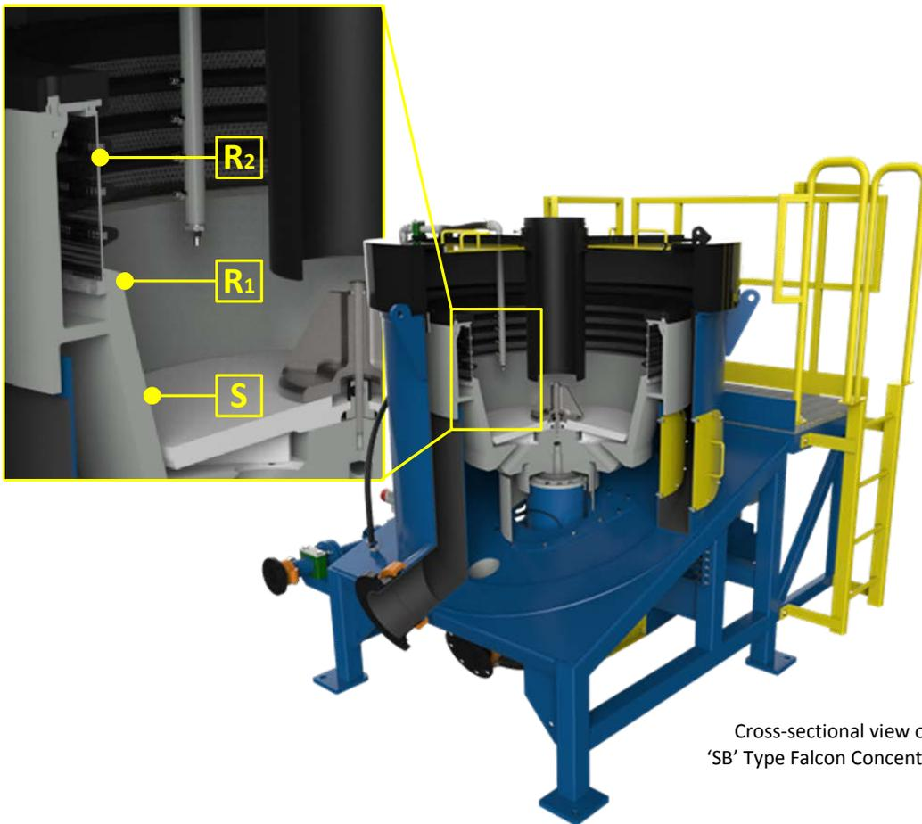
Cross-sectional view of the 'SB' Type Falcon Concentrator
