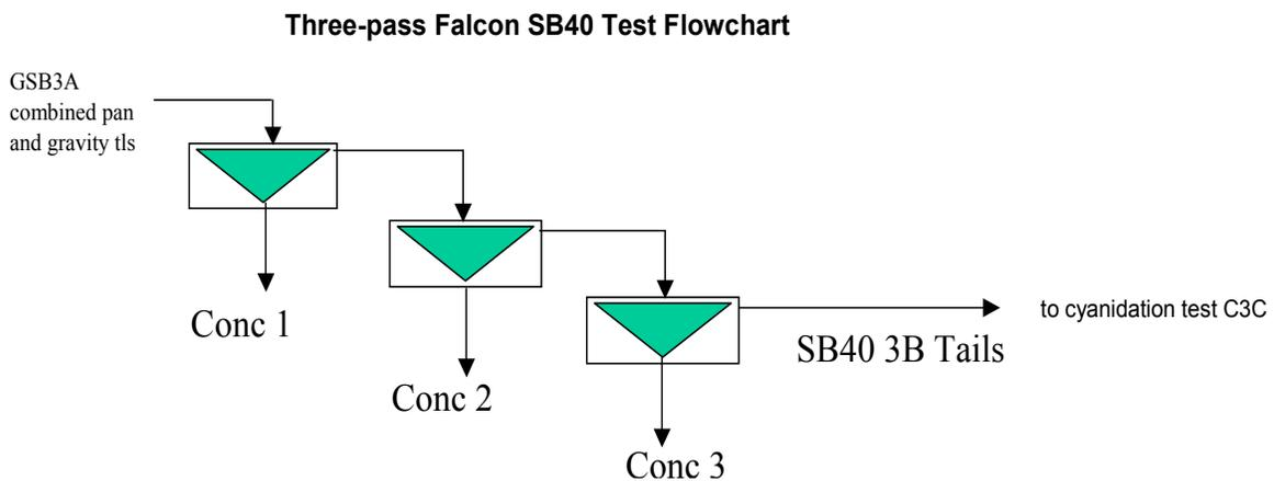
The following chart summarizes the three-pass gravity concentration step. The  $P_{80}$  of the sample after grinding was 65 microns.
