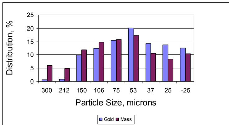
**Graph 4. PSD and Au department in 2<sup>nd</sup> pass – Sulphide sample**
