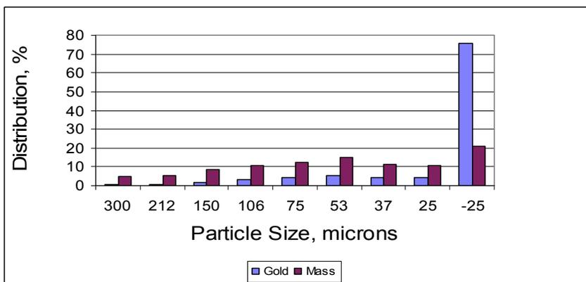
**Graph 2. PSD and Au department in 2<sup>nd</sup> pass – Oxide sample**
