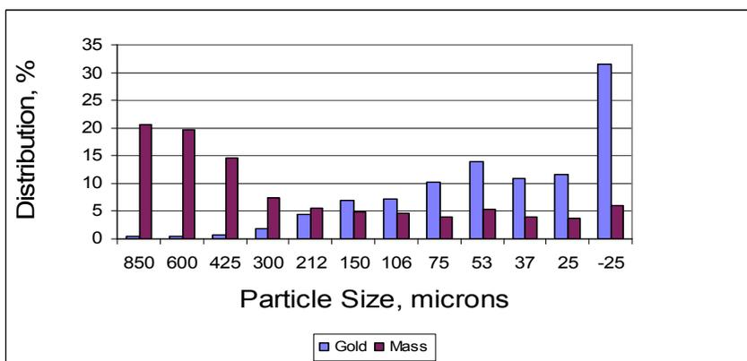
**Graph 1. PSD and Au department in 1<sup>st</sup> pass – Oxide sample**
