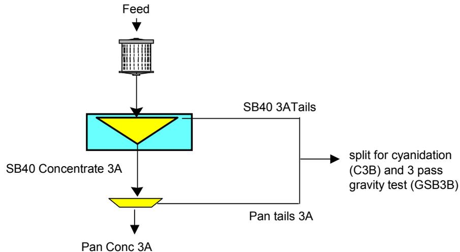
The following chart summarizes the gravity concentration step. The  $P_{80}$  of the sample after grinding was 65 microns.
