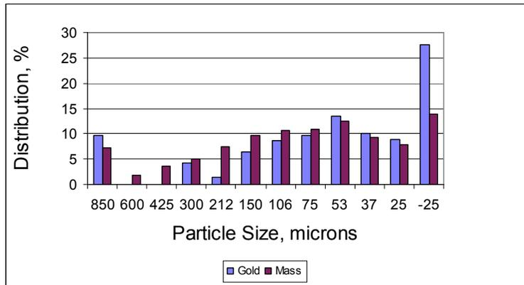
**Graph 3. PSD and Au department in 1<sup>st</sup> pass – Sulphide sample**
