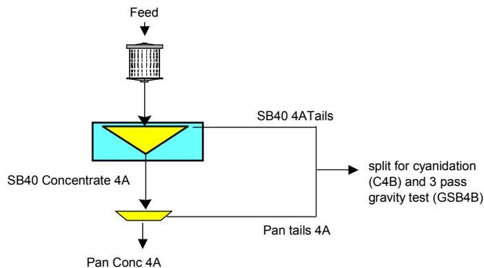
The following chart summarizes the gravity concentration step. The P<sub>80</sub> of the sample after grinding was 68 microns.
