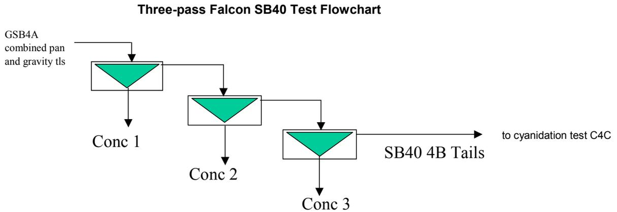
The following chart summarises the three-pass gravity concentration step. The P<sub>80</sub> of the sample after grinding was 68 microns.
